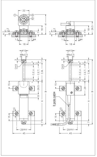
Important: all the data reported in the catalogue linearity, lifetime, temperature coefficient are valid for a sensor utilization as a ratiometric device with a max current across the cursor lc  $\leq$  0.1  $\mu$ A.
